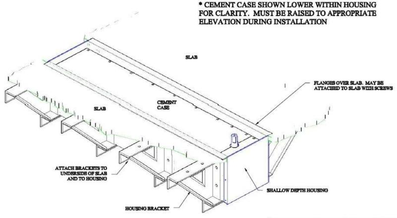
\* THIS IS AN OPTION ONLY. SITE CONDITIONS WILL DICTATE STRUCTURAL REQUIREMENTS. HOUSING MUST BE ADEQUATELY SUPPORTED FOR DOWNLOAD & LATERAL LOAD.
