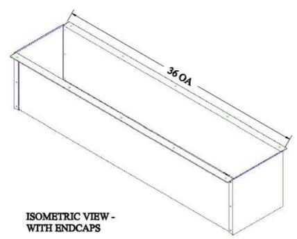
NOTE: RIVET ENPLATES TO HOUSING SIZES VARY BY STRUCTURAL CONDITIONS
